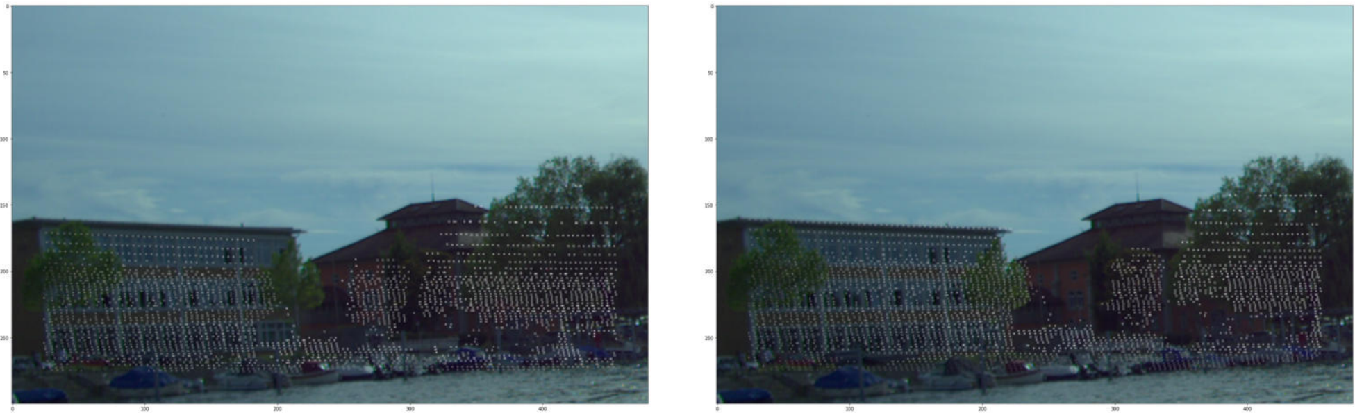
Fig. 4. Visualizing projected Lidar data points in the image plane of the camera: Unregistered (left) and registered (right).
